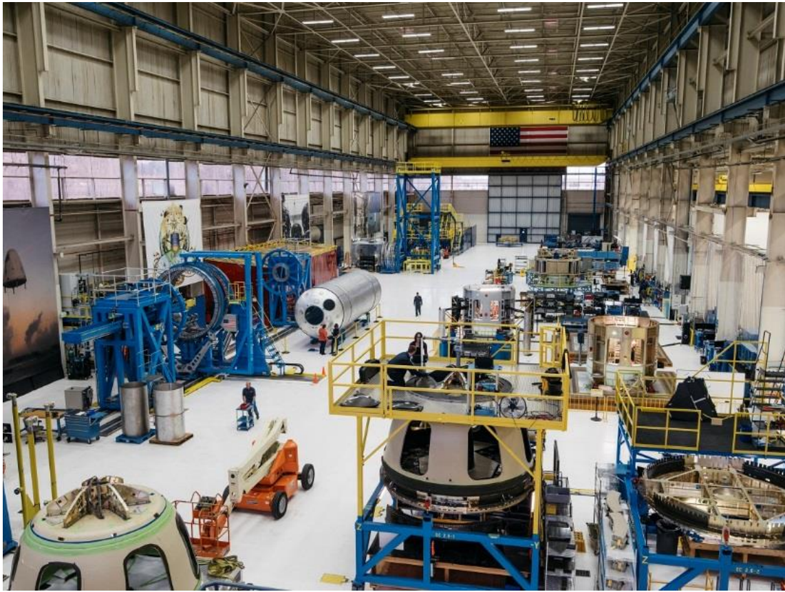
New Shepard spacecraft take shape on the assembly room floor at the Blue Origin plant outside Seattle, Washington. Reproduced by permission of Blue Origin.
